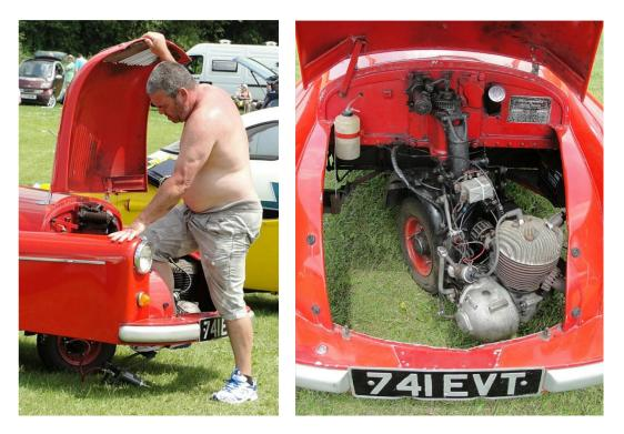
This is not only the way to pump up a Bond front tyre, but also how it has to be kick-started. The engine also turns with the steering!
